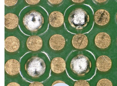
Solder ball size \Phi 600\mu\text{m}
